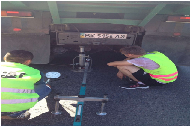
Figure 7 – Measurement of elasticity modulus of road pavement with plate equipment “Infratest”, 2016
