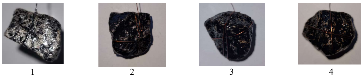
Figure 1 – General view of representative samples of granite crushed stone after testing: 1 (base bitumen BND 70/100), 2 (bitumen with 0.3 % Adbit-R), 3 (bitumen with 0.4 % Adbit-N), 4 (bitumen with 0.5 % Adbit-N)
