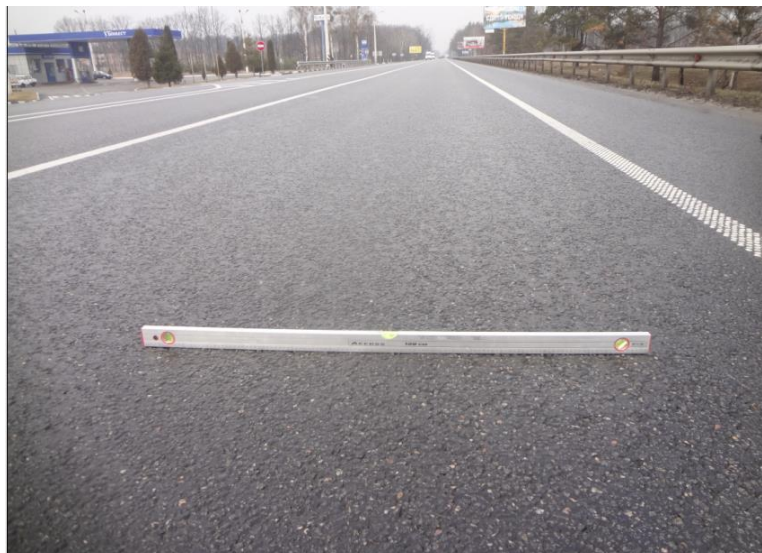
Figure 9 – Lack of rutting on a straight section
