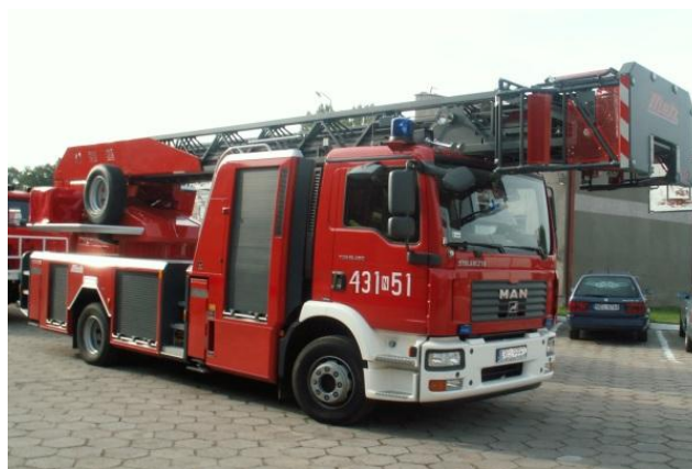
Rys. 2. Autodrabina MAN - METZ SD 32 [4]
