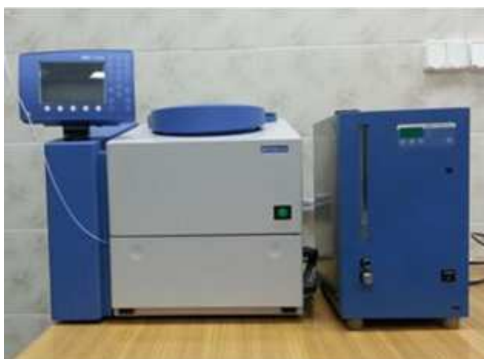
Figure 1 – IKA C5000 calorimeter used in measuring the heat of combustion
