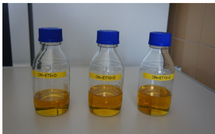
Figure 3 – Mixture of diesel oil with 5%, 10% and 15% of ethanol by volume and 2% dodecanol addition
