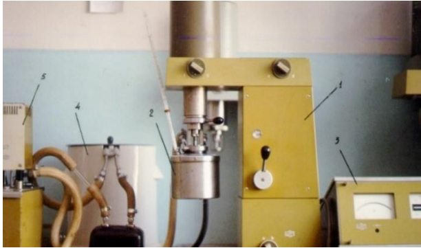
Figure 4 – General view of the rotational viscometer REOTEST 2.1
